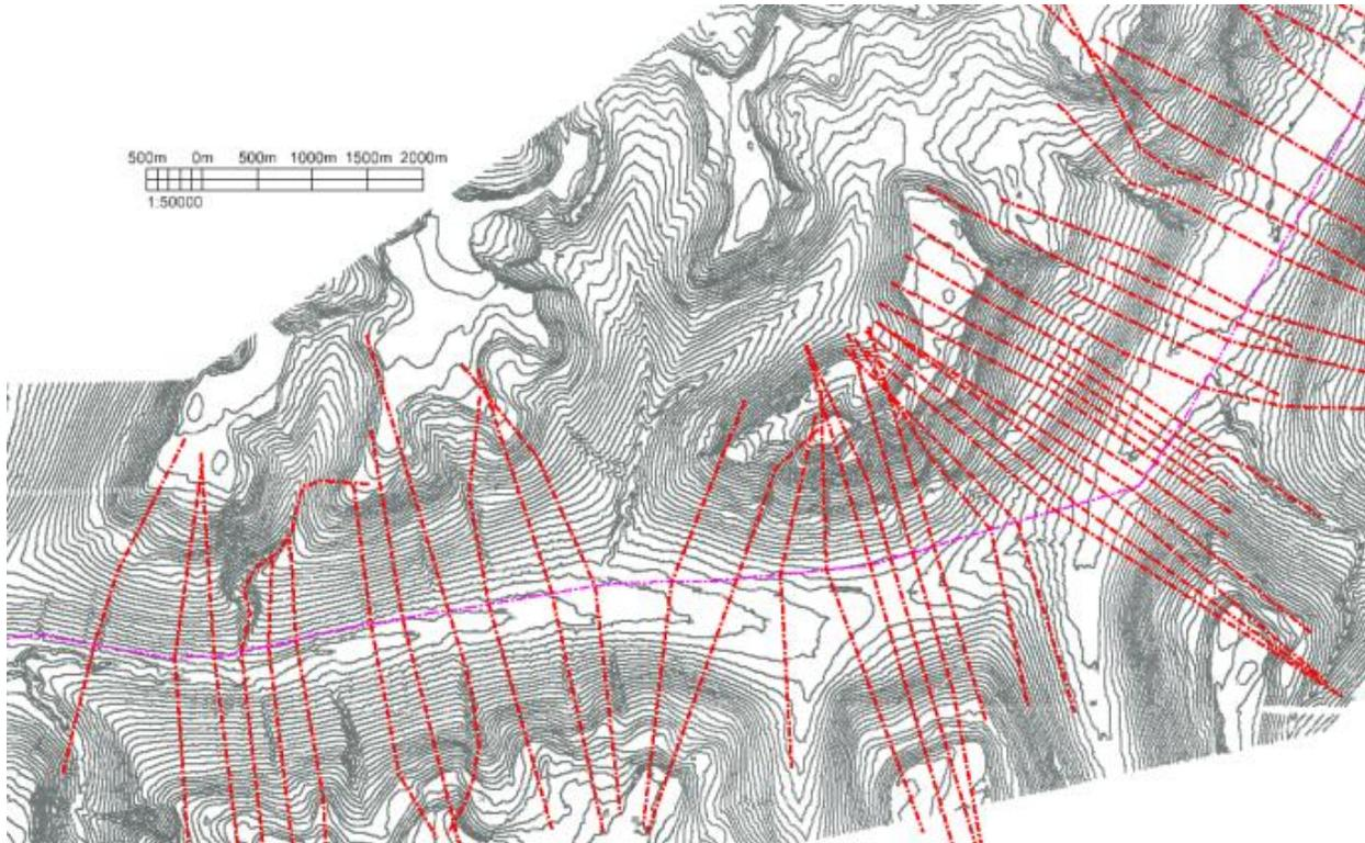
Figure 2. The figure shows the transmission line over Öxnadalsheiði pass. Pattern lines (cross sections) cross the transmission line, from mountain top to mountain top.
