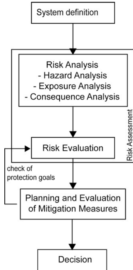
Figure 1: Schematic workflow of a risk-based decision process as it is implemented in EconoMe-Develop
