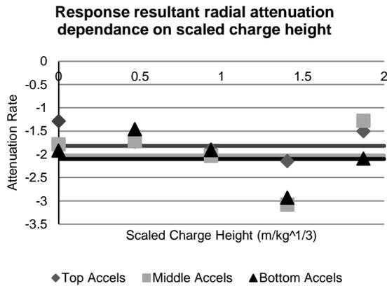
Figure 6: Radial attenuation rates (d) dependence on charge height. The horizontal lines represent the average attenuation rate for each accelerometer depth.
