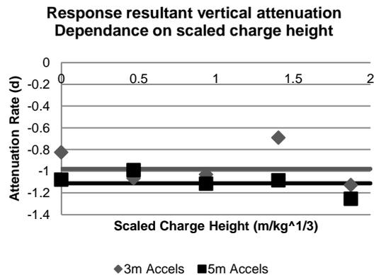
Figure 7: Vertical attenuation rate (d) versus scaled charge height with averages for the individual data series shown by solid horizontal lines.
