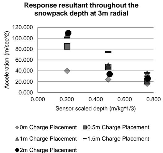
Figure 3: Average peak acceleration responses 3m radially from the charge center verses scaled sensor depths for various charge heights.
