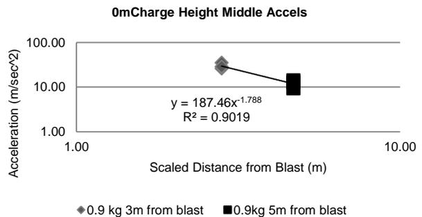
Figure 5: Acceleration magnitudes recorded at the middle snow layers for multiple charges placed on the snow surface. In this case, c=187.46 and d=-1.788.
