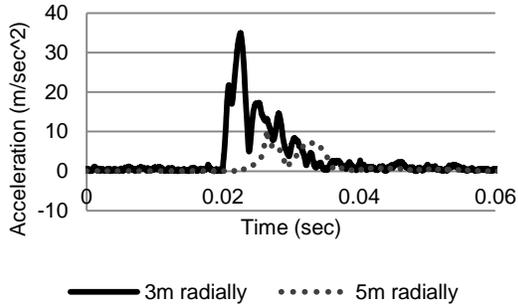
Figure 2: Example resultant acceleration magnitude data 3m and 5m radially from the charge. The resultant acceleration is the vector magnitude comprised of the vertical and radial acceleration components. Each data series is the acceleration magnitude of a single dual axis accelerometer experienced.
