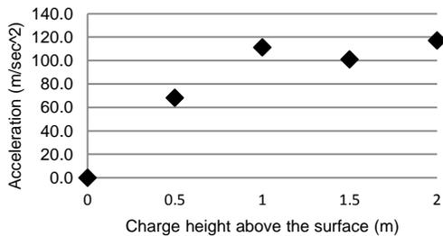
Figure 4: Percent increase over surface placement in average acceleration experienced in the top layer of snow for various charge heights at a distance of 3m from the explosive.
