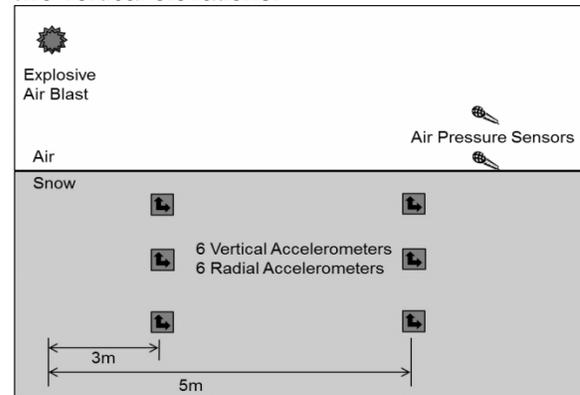
Figure 1: Typical test set up with accelerometers at two radial distances, three snow depths, and two air pressure sensors.
