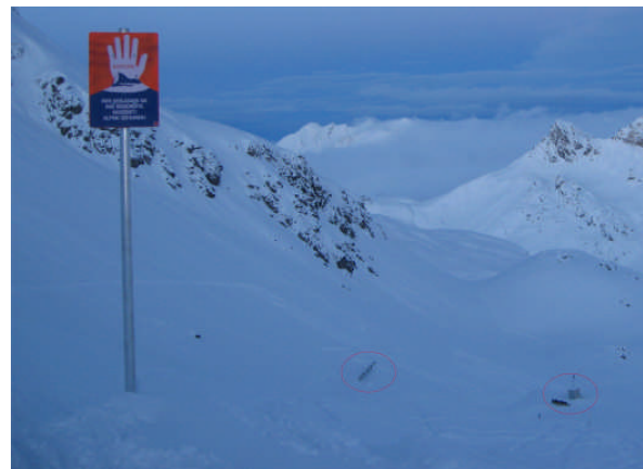
Figure 1. The Snowcatcher test site. Red circle middle: test net system, right: measurement shelter.
