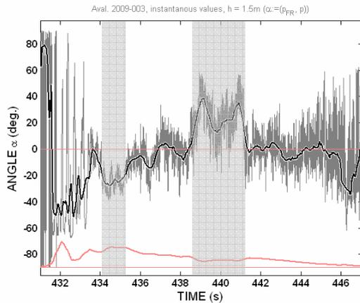
**Figure 8:** Instantaneous orientations of the resultant force at  $h=1.5$  m in avalanche 2009-03. The red curve is the pressure measure by the cantilever sensor.
