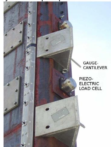
**Figure 2:** Piezo-electric load cell are installed on the hillside of the VldS pylon. They have an area of  $80 \text{ cm}^2$  (diameter 10 cm).
