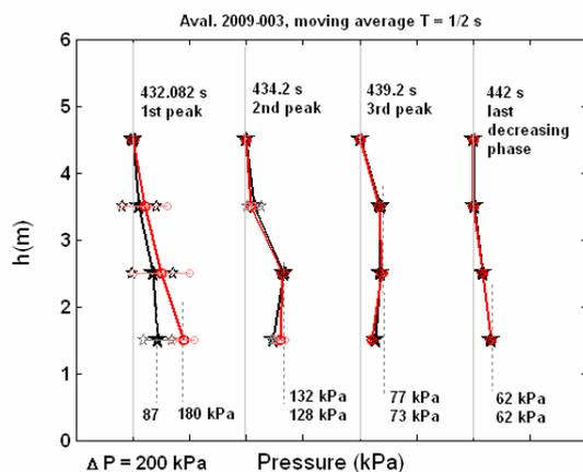
**Figure 7.** Evolution of the impact pressure profile at few characteristic times. Piezo-electric (black) and the cantilever-sensor (red). Horizontal bars are one standard deviation.
