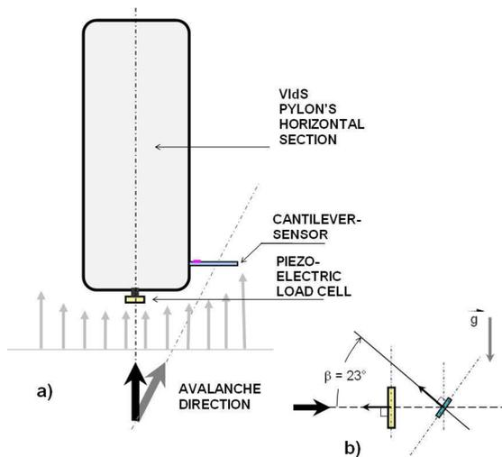
**Figure 1:** a) Pylon section indicating the position of the sensors. b) There is an angle of 23 degrees between the surfaces of the piezo-electric load cell (left) and cantilever-sensor (right).
