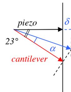
**Figure 5.** Load deviation angle,  $\alpha$ , from the surface orientation of the cantilever sensor, and resulting difference,  $\delta$ , in the pressure measured by the two sensors.
