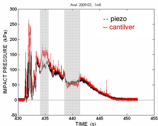
**Figure 6.** Avalanche 2009\_003. Impact avalanche pressure measured at 1.5 m above ground by piezo-electric (red) and cantilever-sensor (black).
