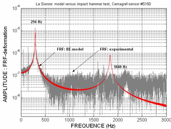
**Figure 4.** FRF of deformations of the cantilever sensor as given by *in-situ* impact hammer test (black) and Bernoulli-Euler beam model (red).
