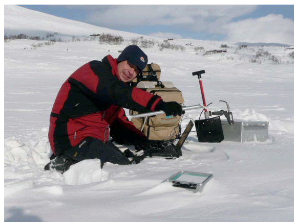
Figure 3. Measurements of spectral reflectance of the snow surface with the 'Analytical Spectral Devices Fieldspec Pro spectroradiometer' on Breiddalsvatnet, March 5 th , 2009. Measurement results are presented in Figure 5.
