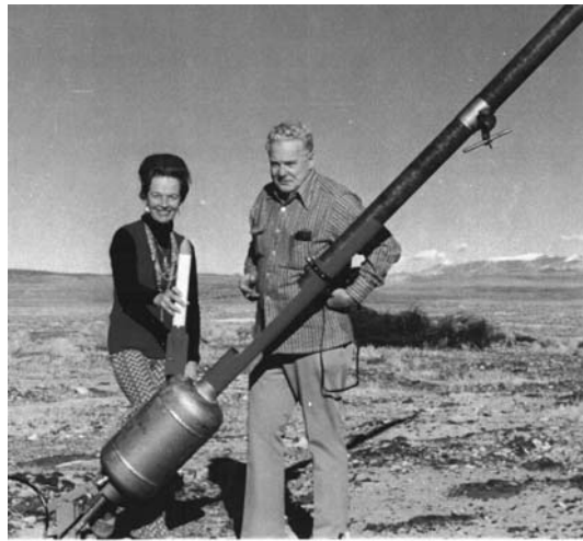
Figure 4. Jerry and Monty in 1974 with an MK 16 launcher. The projectile utilized three cast primers, each weighing 350 grams. Photo courtesy of Pete Peters.
