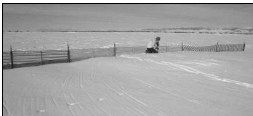
Figure 6. Measuring drift depth along center line.
