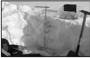
Figure 9. Conducting a cross-sectional analysis of snowpack at drift apex.
