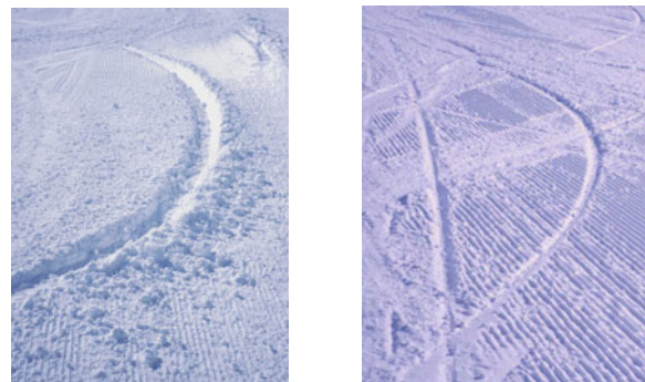
Figure 8. Effect of time on snow hardening by sintering. Left: 2 hours sintering, right: 10 hours sintering.
