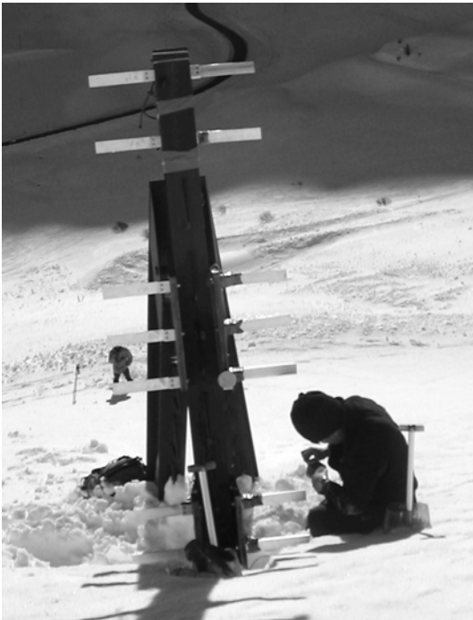
Figure 2: Aluminium targets on the tripod
