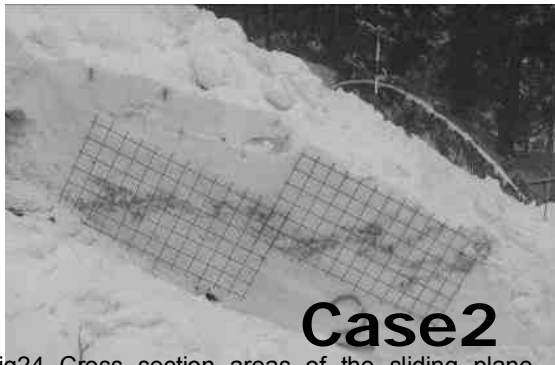
Fig24 Cross section areas of the sliding plane zone after detonation for case 2
