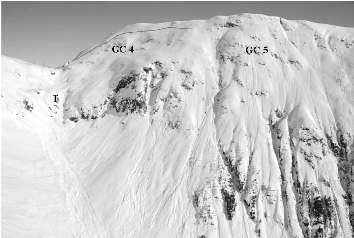
Figure 2: The location of the avalanche fracture line on Path GC4 above the Tower 113 location (T). The fracture lines of March 28 would also extend across GC5.
