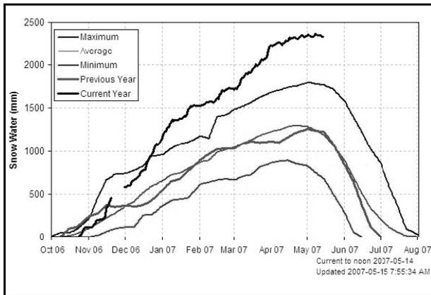
Figure 3: Snow pillow data 2006-2007 Tahtsa Lake (Station 1B02; elevation 1300 m). Source: BC Ministry of Environment, Water Stewardship Division.
