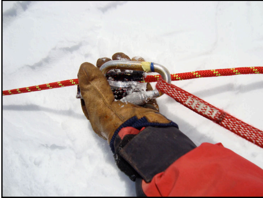
Figure 2. Petzl Shunt on fixed rope
