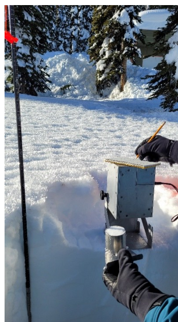
Figure 6: The IRIS displayed in use in a snow pit, with the collection cylinder showing the layer of snow of interest.
