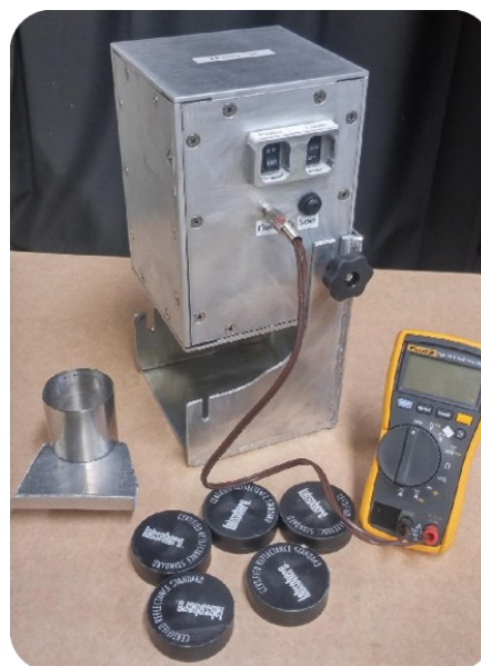
Figure 5: The IRIS displayed along with the calibration discs, collection cylinder and the multimeter used to display the recorded reflectance value.
