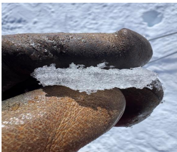
Figure 6: Photo showing bed surface made up of buried near-surface facets above a thin melt-freeze crust from Figure 5 avalanche.
