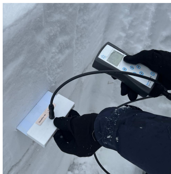
Figure 2: Using the SnowPro 25 inserting it into the side wall of the pit. (Photo: Robyn Gotz, Montana State University, 17 April, 2026)
