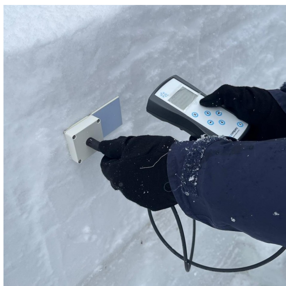
Figure 1: Example of how we placed the SnowPro 17 on the side wall of a snowpit while performing measurements. (Photo: Robyn Gotz, Montana State University, 17 April, 2026)
