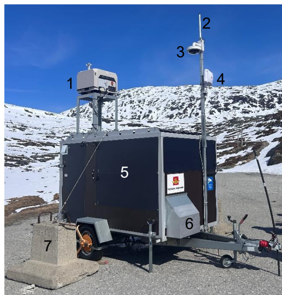
Figure 1: Mobile drone station set up: 1) Drone station (DJI Dock 2/3). 2) Airspace surveillance system. 3) 360°webcam. 4) Mobile cellular network antenna. 5) Solar panels cover trailer walls and roof. 6) Diesel generator exhaust and air-cooling outlet. 7) Weight to prevent overturning.
