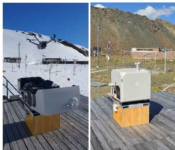
Figure 1: DJI Dock 3 installation on the roof of the small building at the Weissfluhjoch research site.
