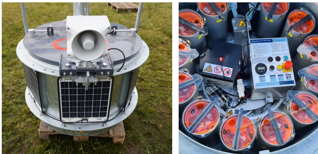
Figure 7: A fully loaded deployment box of a Wyssen LS12 avalanche tower with an additional signal horn installed to warn people and animals in the avalanche's path.
