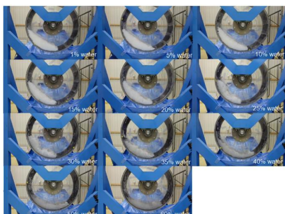
Figure 2A. LWC_M trends for Experiments 5–8. Experiments 5 and 7.1 followed snow-first procedures where LWC_M increased as water was added to snow. Experiments 6, 7.2, and 8.2 followed water-first procedures where LWC_M decreased as snow was added or water was removed. Figure 2B. Experiment 5 snow-first sequence. Water was added from 1% to 60% of the initial snow mass.
