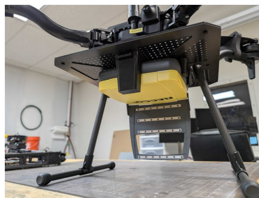
Figure 1: RECCO R9 integrated onto a proprietary payload adapter mounted onto the underside of a drone.
