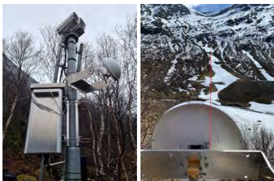
Figure 1: Antenna and box of the 10 GHz Pulse-Doppler-radar (left) and view on to the avalanche track (right).
