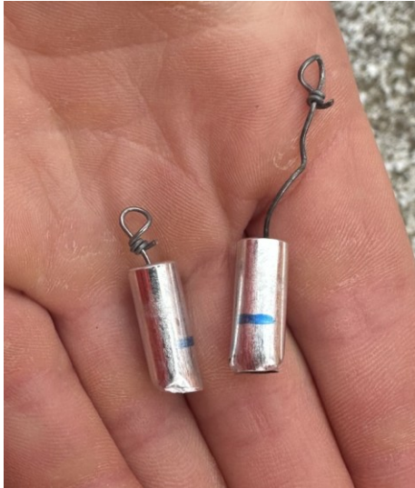
Figure 3: Broken pull wires resulting in a mislight.
