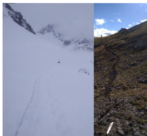
Figure 2: Geometry of the Fiber optic (FO) cable in the field: Right: deployment of the FO cable in the ground; Left: deployment of the FO cable in snow.
