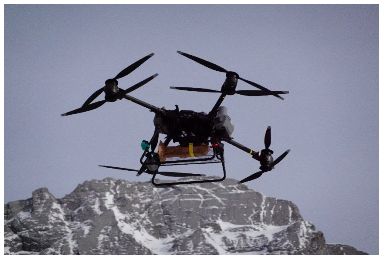
Figure 2: A DJI FlyCart 30 fitted with the AVSS Precision Avalanche Management System (PAMS) in flight.
