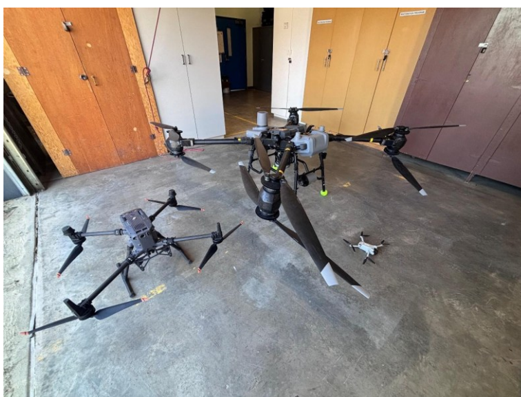
Figure 3: The Jasper Visitor Safety fleet: the heavy-lift DJI FlyCart 30 (Centre), the DJI Matrice 350 RTK reconnaissance aircraft (left), and the DJI Mini training aircraft (right).
