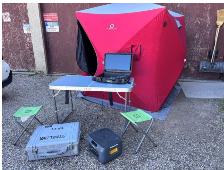
Figure 4: The portable command center: an insulated ice-fishing tent, folding table and stools, an additional monitor, a repackaged Starlink terminal, and a battery box for off-grid operation.
