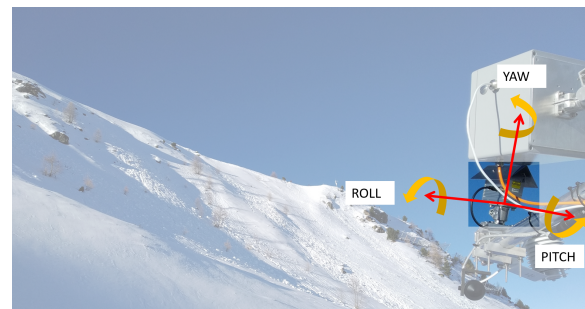
Figure 3: Visualisation of the rotation angles of the scanner, in its own coordinate system.
