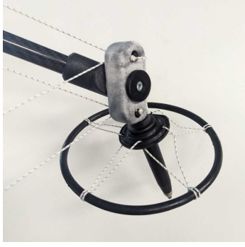
Figure 3: Foot design which allows taking off and landing on snow
