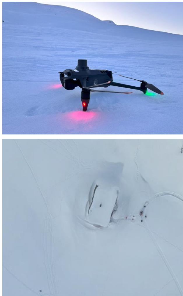
Figure 2. Upper panel: DJI Mavic 3E RTK drone with integrated optical camera. Lower panel: Typical optical imagery gained by consumer-grade UAVs.
