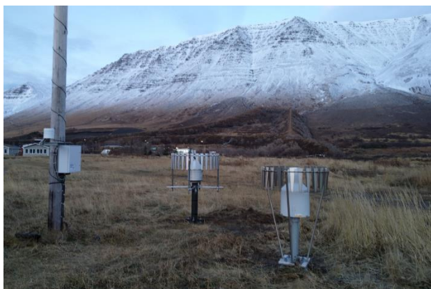
Figure 1: The weather station with two weighing bucket gauges and precipitation sensor in Flateyri , Iceland.
