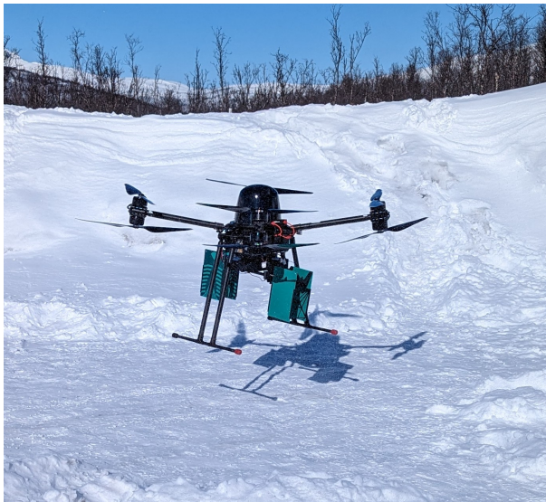
(c) Complete radar system mounted on Cryocopter FOX.
