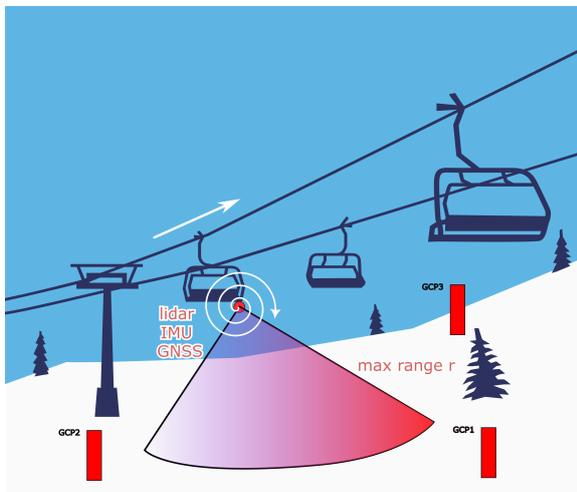
Figure 1: Concept of the setup, where GCPs stands for ground control point (modified from a draft submitted to the Journal of Glaciology Dikic et al. (2024)). A small rotating lidar (10 to 20Hz) is mounted on a gondola or chair. As the lift moves up and/or down, point cloud data is collected and then post-processed with a SLAM algorithm to produce a cumulative point cloud. Subsequently, the snow-free point cloud is subtracted to determine the snow depth.
