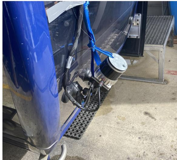
Figure 2: MOLISENS system mounted on the Sonnblick cable car (Goelles et al., 2022; Dikic et al., 2024)
