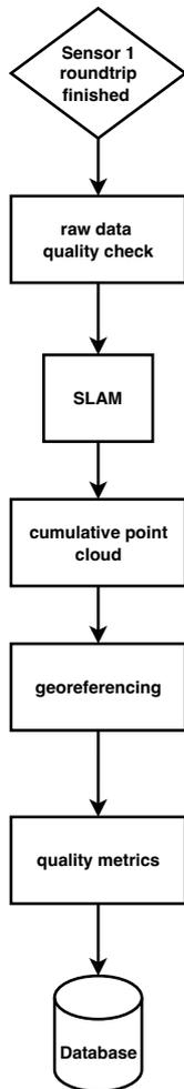
Figure 4: Processing pipeline of a moving lidar sensor.
