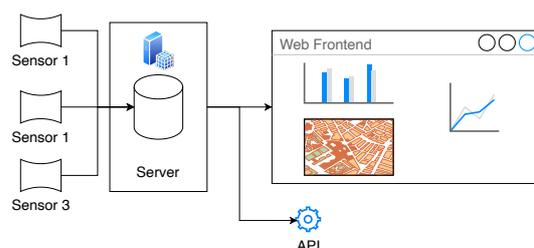
Figure 3: Architecture with multiple sensors and the user facing frontend and an API for integration with other services.
