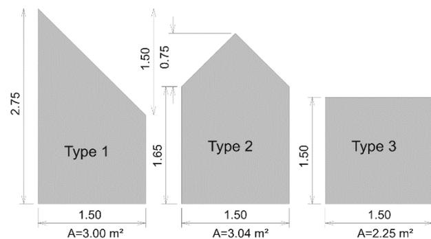
Figure 3 show three types of concrete foundations for barrier posts. Fig.: HNIT Verkfræðistofa.
