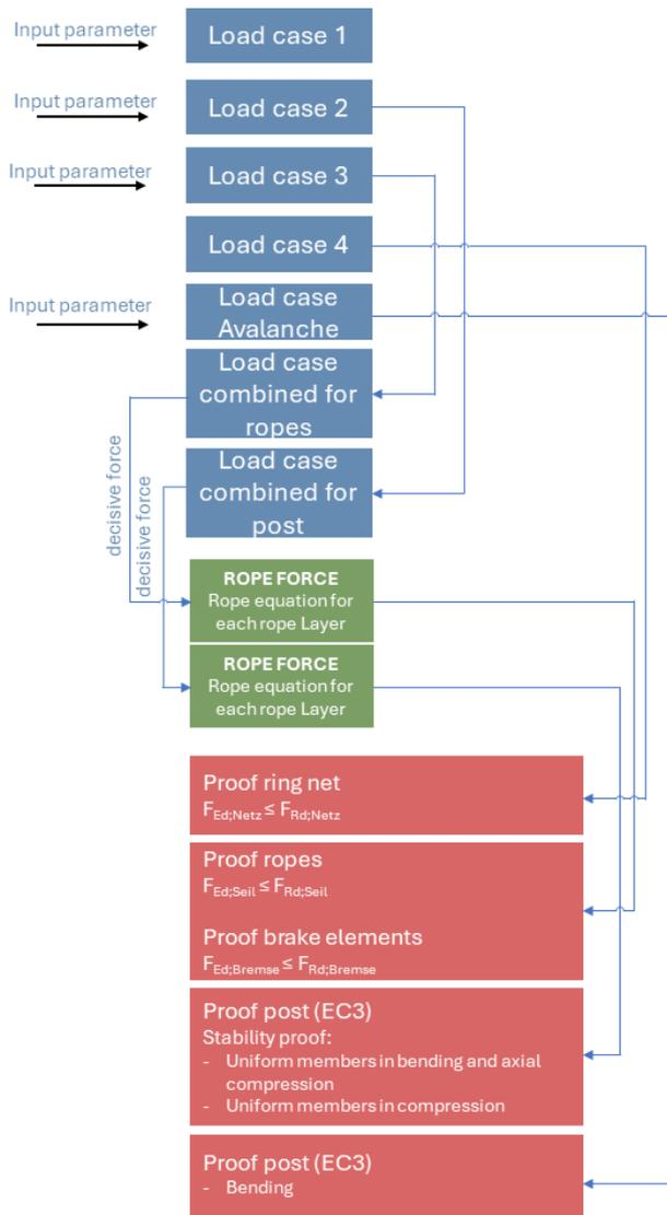
Figure 4. Flow chart for flexible slush flow barrier design calculation (Geobrugg AG, 2024). Fig.: Geobrugg AG.
