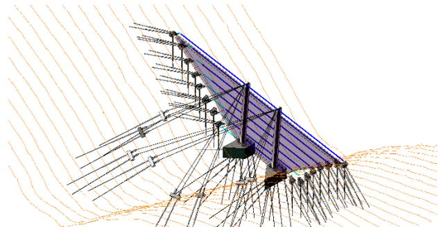
Figure 5 shows a 3D view of typical sub- and superstructure, i.e. retaining ropes, net, ropes, posts, concrete foundations and the anchoring system. Orange lines illustrate the terrain surface. Flow direction is from left to right. Fig.: HNIT Verkfræðistofa.
