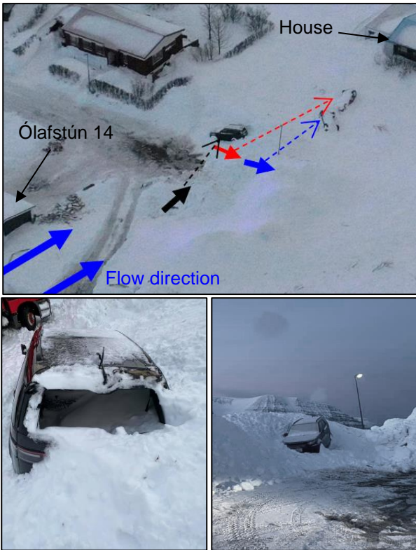
Figure 6: Photos of the three cars after the event. Top: A schematic diagram of the cars' displacement. The two smaller cars (blue and red) were transported 15 m and 20 m, respectively. Bottom: The truck. Photos: K. M. Hákonardóttir and E. Ólafsson.
