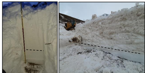
Figure 3: The avalanche debris at the Skollahvilft dam. Left: Type 2 deposit on the lee side of the dam. Right: Type 1 deposit upstream of the dam. The dashed lines indicate the boundary between old snow and deposited snow. Photos: Ó. Hilmarsson.
