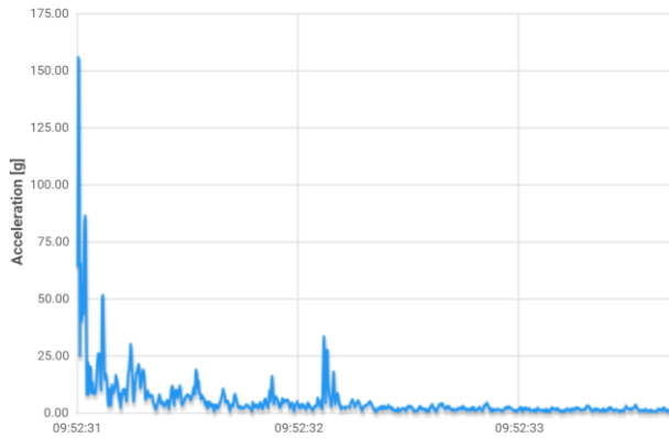
Fig. 16: Corresponding response spectrum of the GUARD's accelerometer to the avalanche impact on June 11, 2024, in Rosalba.
