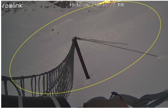
Fig. 12: Recorded snow slide on field 1 on December 19, 2023, at Chant Sura by the real-time monitoring camera "Reolink".
