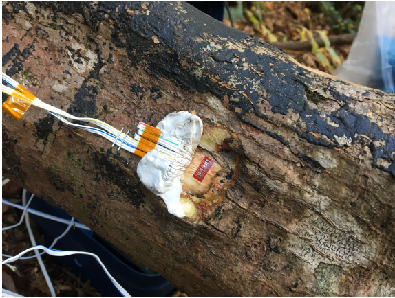
Figure 1: Strain gauges attached on the trunk of tree A.
