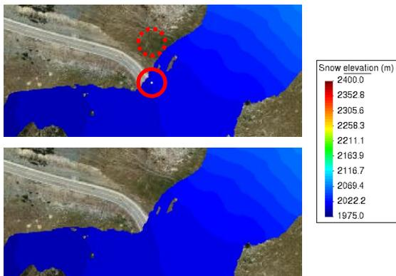
Figure 4: Bonaigua. Map of maximum snow elevation: LiDARv1 (upper) and LiDARv1\_fs (lower). Values lower than 1975 m are represented in white (highlighted in a circle).
