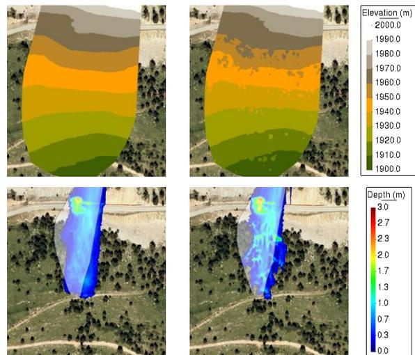
Figure 6: Coll de Pal event simulated with LiDARv1: DEM (upper left) and DTM (upper right); map of maximum depth with topographical data as DEM (lower left) and as DTM (lower right).
