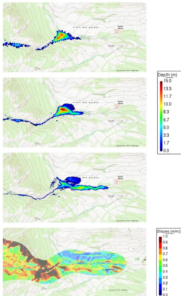
Figure 5: Àrreu. Map of depth when the avalanche stopped (upper maps). Map of slopes (lower map), coloured map filtered from 0 to 1 m/m (black colour represents slopes higher than 1 m/m).
