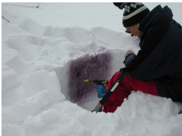
Figure 4: Visualization of the deposit texture by spraying an ink–alcohol mixture onto the vertical face of a snow pit and warming it lightly with a camping-stove burner.
