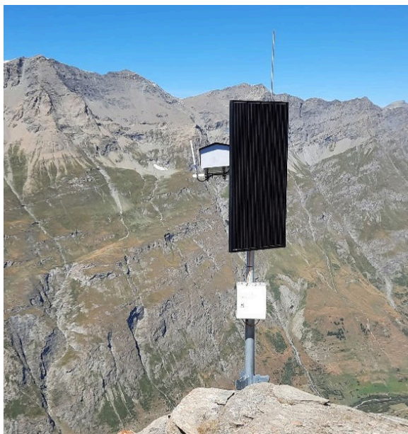
Figure 1: The camera monitoring system installed close to the Pointe du Soliet in Bessans, France, with the avalanche release zones of interest close to the Pointes du Châtelard and Pointe de Claret in the background.
