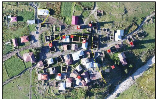
Figure 6 : Location of 1987 main destruction limits inside the village (yellow dashes) from south-facing slopes avalanche – current towers appear in red.
