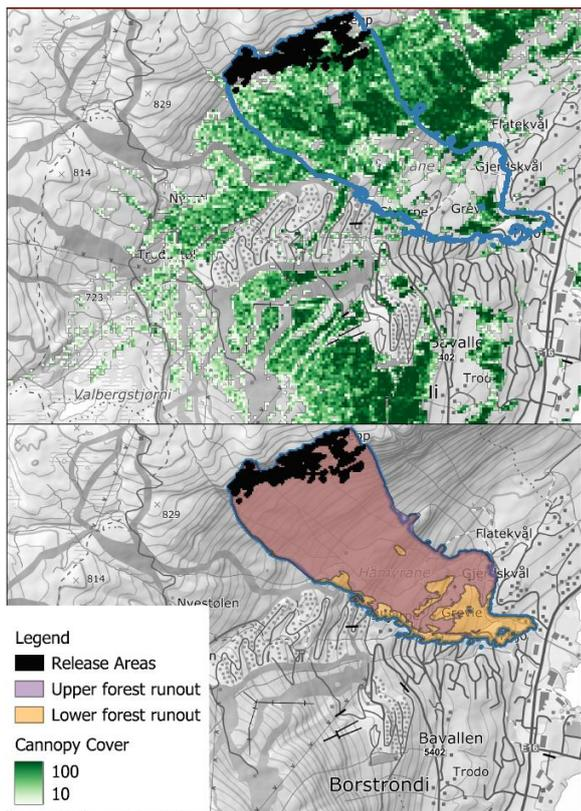
Figure 5: An avalanche path where the errors of predicted forest structure led to a noticeable difference in runout distance. The largest area is outlined in both maps. The access road to the ski resort and some residences are affected by these differences. The base maps are provided by the Norwegian Mapping Authority under CC BY 4.0. © Kartverket
