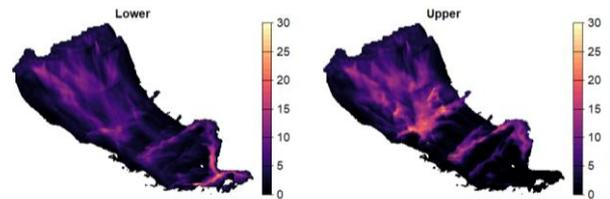
Figure 6 – Height profiles of the simulated avalanche depth (i.e the total of flowing and deposited snow) in the lower and upper forest scenarios showing the braking effect of a dense forest in the runout path.
