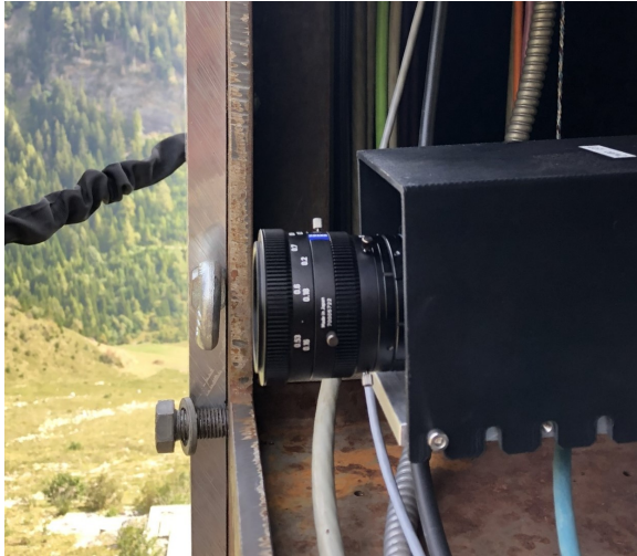
Figure 3: Picture of the camera in its position inside the pylon during assembly. The camera shown is protected by a 3D-printed cover.
