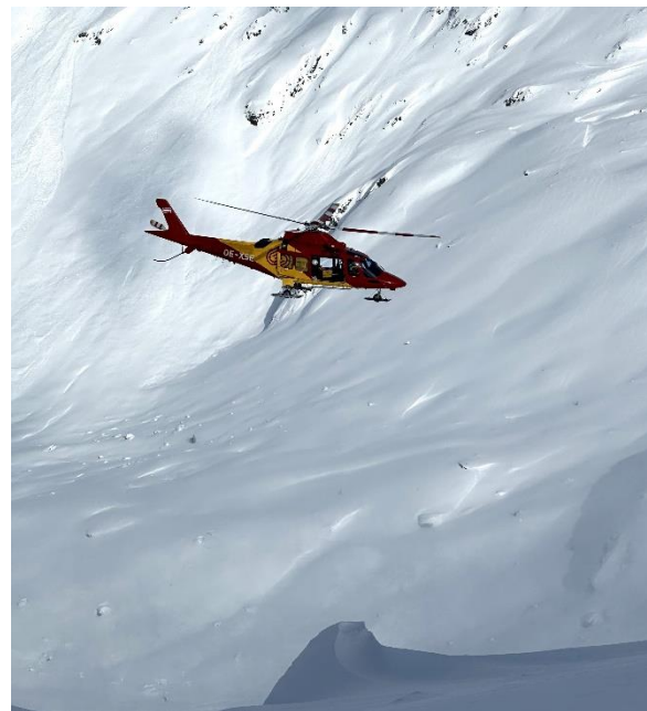
Figure 2: Members of the Idalpe avalanche-safety-team triggering avalanches by explosives with the Schenk Air helicopter permanently stationed in the ski area.
