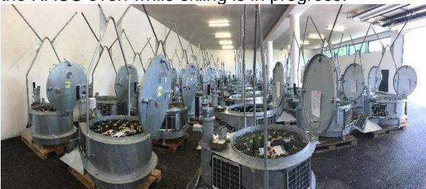
Figure 5: Warehouse between the two bunkers for the deployment boxes of the actually 74 Wyssen avalanche towers from the ski resort and 8 from the municipality of Ischgl.
