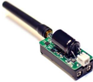
Figure 1: Electronic igniter and communication unit. Photo: AF Decom
