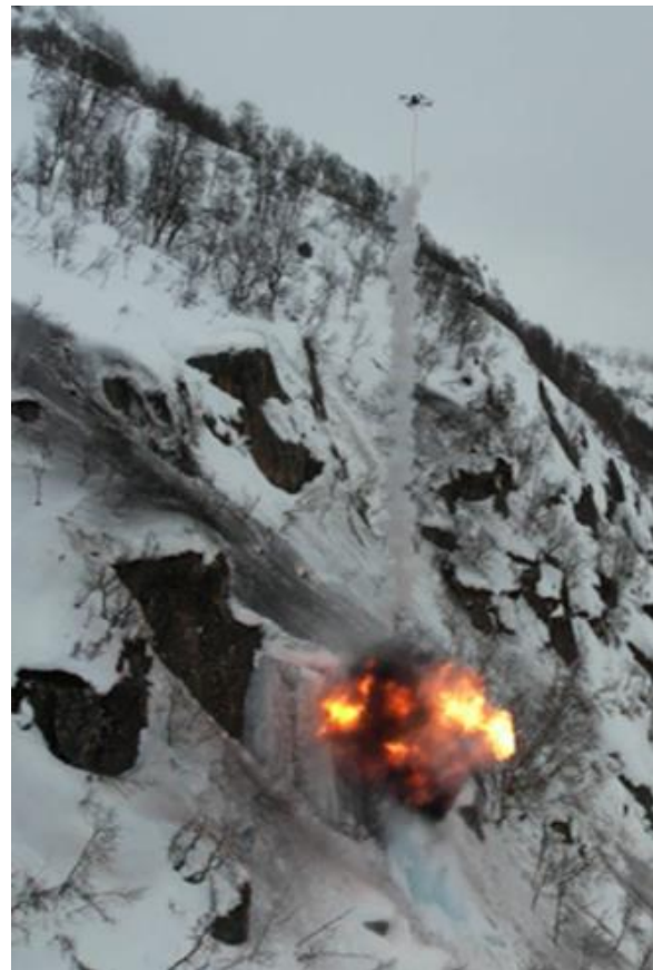
Figure 3: Detonation of 4 kg mix of TNT and RDX hanging on a detonating wire underneath the UAV. Photo: AF Decom
