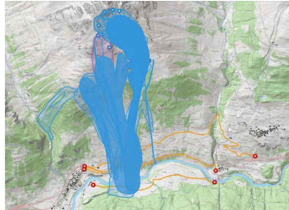
Figure 5: Gonda avalanche path with example set of historic avalanches (blue), closure points (red) and affected infrastructure (road, trail, railway) (orange).
