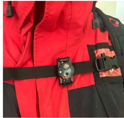
Figure 1: Blast Gauge sensor being worn on the chest strap of an avalanche worker.
