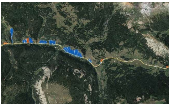
Figure 8: Zoomed in view of avalanche paths on Lizard Head Pass, provided by CDOT
