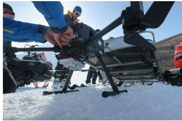
Figure 3: Multispectral camera mounted on UAV.
