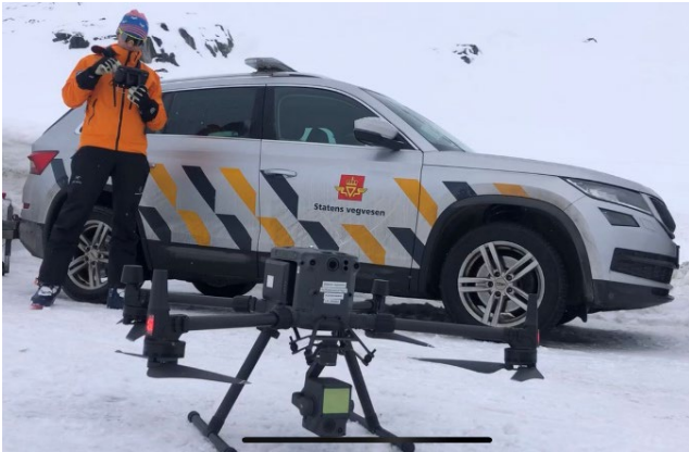
Figure 4: UAV-borne LiDAR scanner preparing for take-off.
