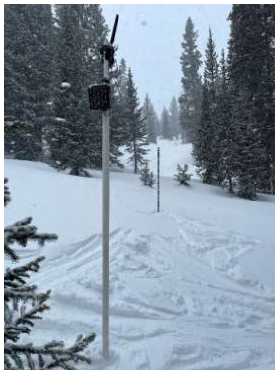
Figure 2: The Purple Ridge game camera monitoring site. In the foreground, the game camera and solar panel are mounted a meter above the snow surface on a PVC pipe. In the background, a PVC with electrical tape is used as a snow stake.
