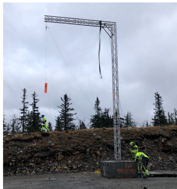
Figure 2 - Temporal tower for testing explosives. Photo: N. Farestveit, NPRA
