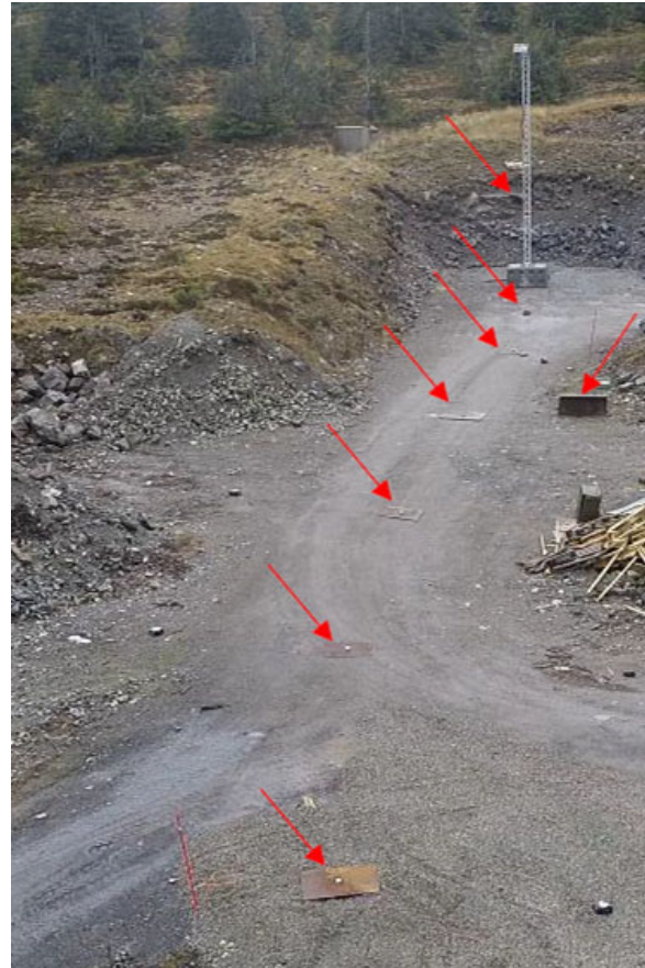
Figure 6 - Overview over the test site. Shock pressure sensors shown with red arrows. Photo: AF Decom
