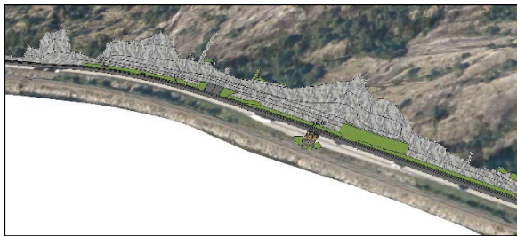
Figure 3: Protective measures will consist of dams blasted into the mountain. Screenshot of 3D-model created by Lars Joergen Sandvik.
